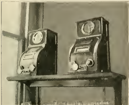
COLEMAN BLOCK SIGNAL INSTRUMENTS, SHOWING PUSH BUTTONS AND UNLOCKING PLUNGER, N. Y. C. & H. R. R.R.
